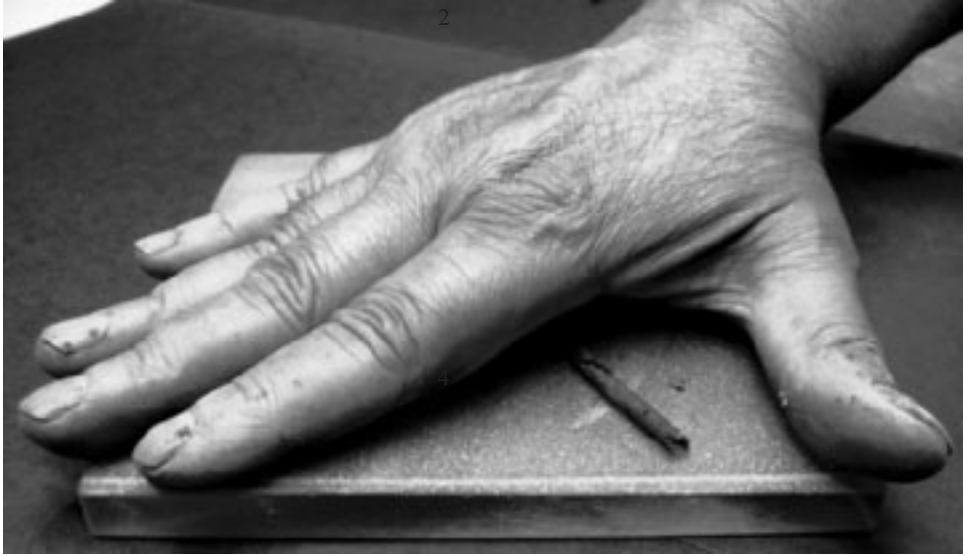
Figure 4.7 Rolling of soil mass on ground glass plate to determine plastic limit (Courtesy of Braja M. Das, Henderson, Nevada)
