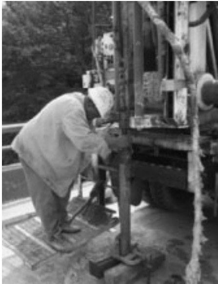
Figure 18.7 Drilling rod with split-spoon sampler lowered to the bottom of the borehole (Courtesy of Braja M. Das, Henderson, Nevada)
